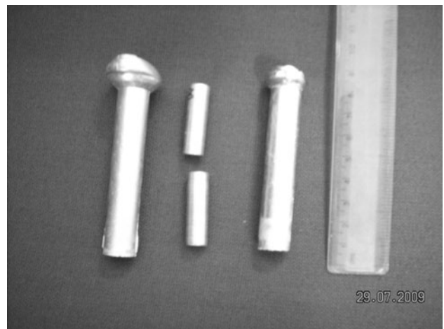
Fig. 3 Photograph of composite casting and pins
