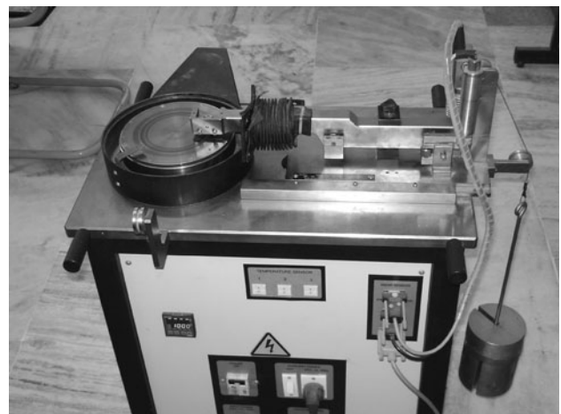
Fig. 4 Photograph of pin-on-disk apparatus
